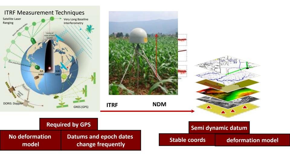
Semi dynamic datums are aligned with the ITRF Coordinates transformed reference epoch using the national deformation model
