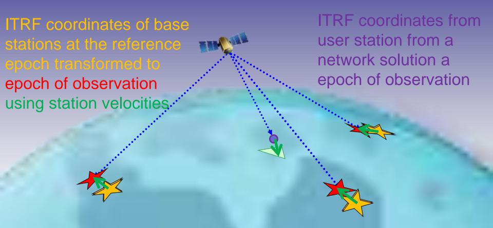
ITRF coordinates need to be projected from epoch of observation to the reference epoch using NDM
